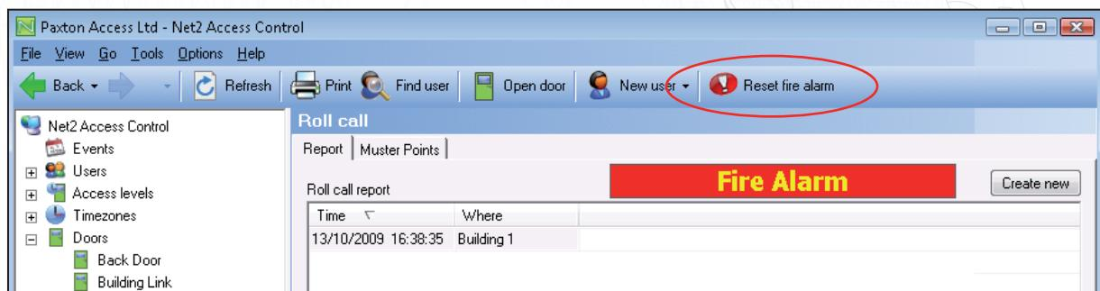
Resetting the actual fire alarm itself will NOT reset this condition or relock the doors. Unless the 'automatically reset fire alarm' feature is enabled.
